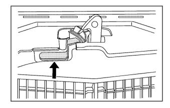
Then go to the front of the vehicle and find the secondary hood release lever. The lever is located under the front edge of the grille near the center. Push the release lever up and raise the hood.
